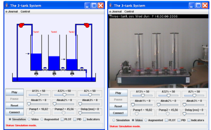
Fig. 5. Two views of the remote lab for level control of a three-tank system.
