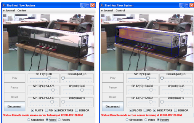
Fig. 4. Two views when the real didactical setup is used for experimentation instead of the model. The view on the right shows how the 3D representation of the heat-flow apparatus is overlapped to the view as an augmented reality technique to improve the user perception.
