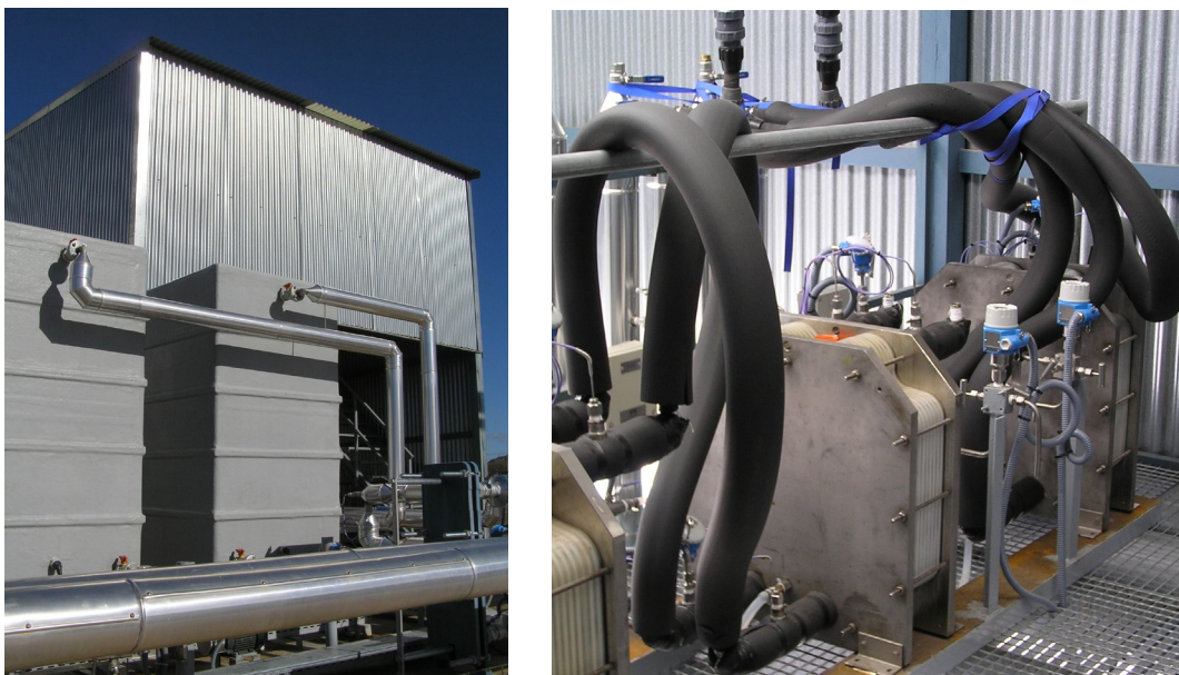
Figure 2. MD Pilot plant at PSA facilities (left) and Scarab AB membrane distillation modules used in the experimentation (right).
